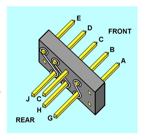
The finished adapter now has four pins out the rear and five out the front. Clean the unit of excess soldering flux if necessary, using a toothbrush and rubbing alcohol.
