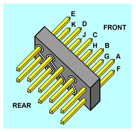
Cutting as close to flush with the plastic header as possible, trim off the front end of the entire front row of pins F - K.
